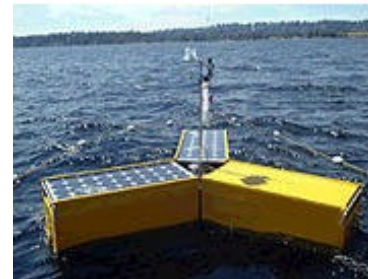
Fig. 6: Sensor-based monitoring system (RUSS, Apprise Technology Inc.) in use at Rensselaer's Darrin Fresh Water Institute
