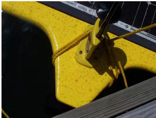
Figure 11. Bio-fouling on vehicle shell: day 11
